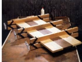
These clamps offer wooden bars with a specially milled, everso-slight radius that distributes downward pressure evenly over the entire surface of the glue-up as the metal jaws (attached to a scissors-like mechanism) squeeze the boards inward. No more bowing or cupping!
