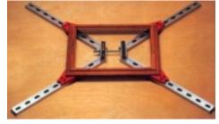
These are also fairly inexpensive, can be used for picture frames or cabinet door assembly and can often accommodate a wide range of project sizes.
