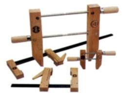
Typically made of hardwood with steel bars, they work with an eccentric cam-type tightening mechanism and offer protective cork jaw pads that also minimize slippage. The larger sizes of these offer throat depths that exceed most bar-type clamps (often up to 6" or more)...a real advantage when you need the added reach for certain types of glue-ups.
