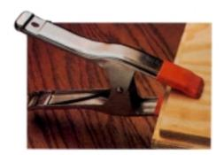
Working much like a clothespin, you merely squeeze the handles together to open the jaws, then release them to clamp your components together. These are normally available in opening capacities ranging from 1" to 3" or 4" and are quite inexpensive.
